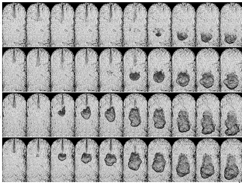
Fig. Visualized results of spray combustion for (E)&(D) blend fuels
